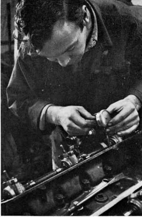
LEFT — Joe Virag checks out the valves with a dial indicator prior to disassembly of the engine. All timing was carefully checked during dismantling and assembly. ABOVE — Ports on exhaust side are huge and virtually straight through. No enlargement necessary but all ports were matched to manifolds and equalized in size.
