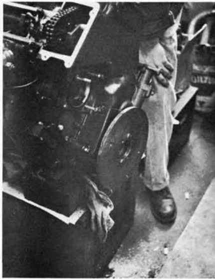
A degree wheel is a must if accurate valve timing is to be achieved on MG.
